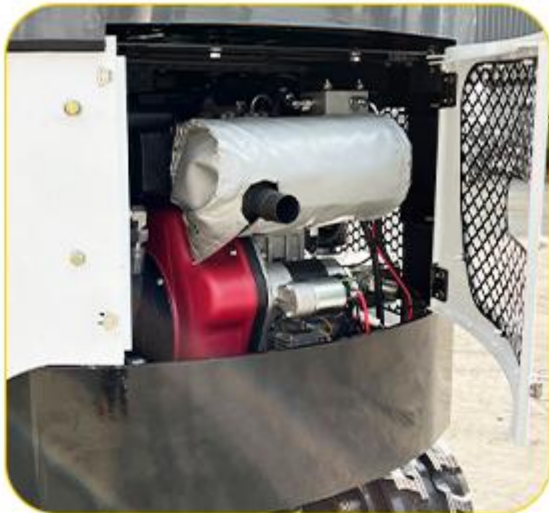
The tail section can be opened for easy maintenance and inspection.
