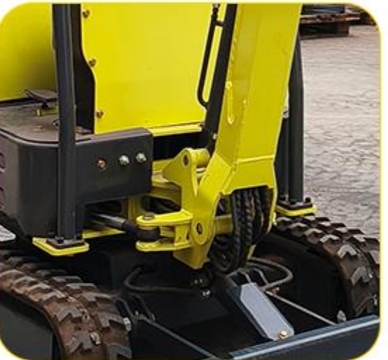
Upper arm lateral swing function
