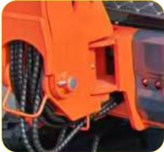
The upper arm can pivot left and right, allowing for more flexible operation.
