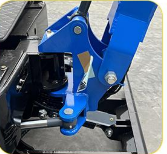
The boom can tilt 60 degrees to the left and right, making operation more flexible.
