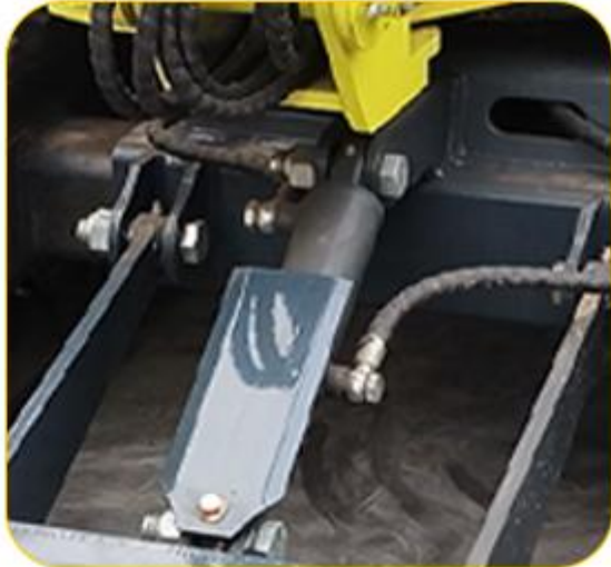
Bulldozing plate cylinder safety coverprotects cylinder rod and pipes.
