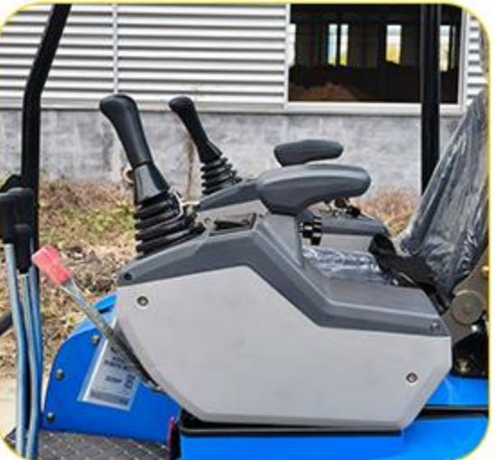
When the control lever is lifted, all operations stop.
