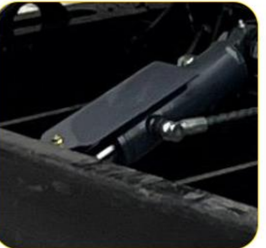
Hydraulic cylinder, pipes protection cover
